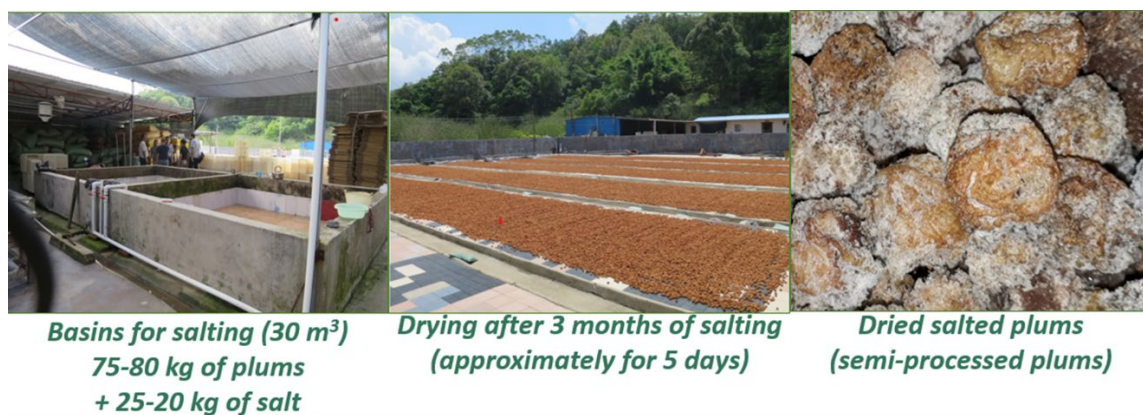
Picture 2: The first step of processing: salting and drying of plums. Salted plums may be the final product or raw material for the production of sweetening plums.
